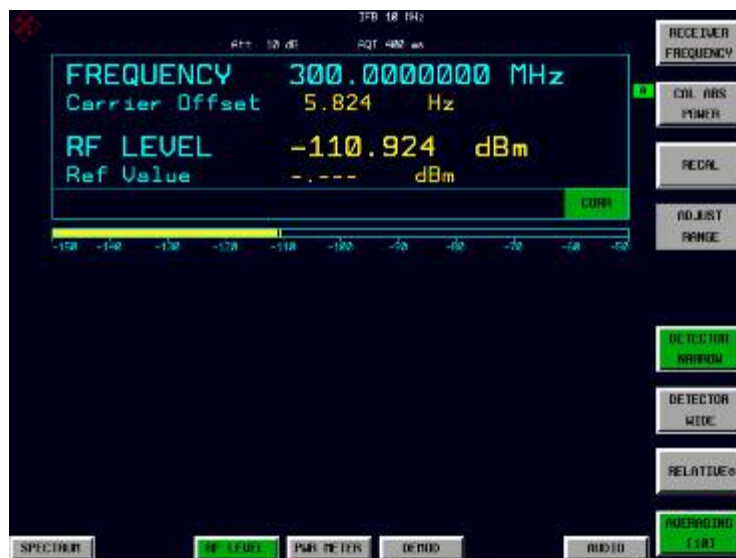
Fig.1-8 Tuned RF Level measurement with Averaging
