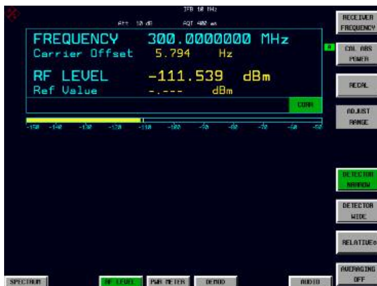
Fig.1-7 Tuned RF Level measurement at low levels
